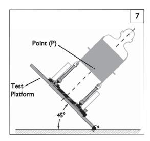
Rear view of wheelchair and human surrogate secured on a test platform and tilted to 45°
